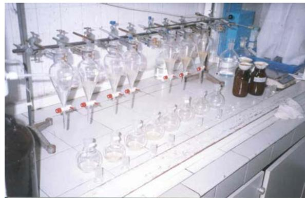
*Pesticides are extracted from soil samples with solvent in a shaker (right) and water is removed using separating funnel.*
