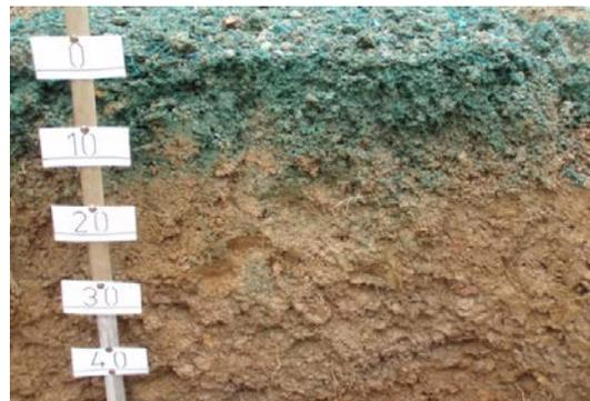
*Excess soils were removed from the hole Dye is seen at all soil layers of the profile*
