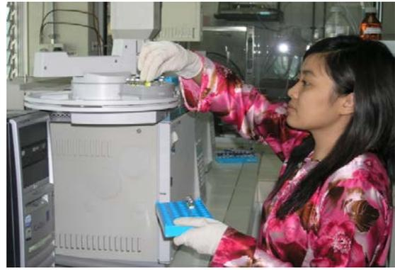
*Highly sensitive and precise instruments such as gas chromatograph are used for pesticide detection*
